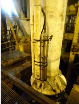
INTEGRipod™ NXT subsea logger strapped to a riser & attached to (Optional) Acoustic Transponder.
