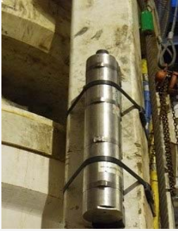
INTEGRipod™ NXT subsea logger strapped to a LMRP.
