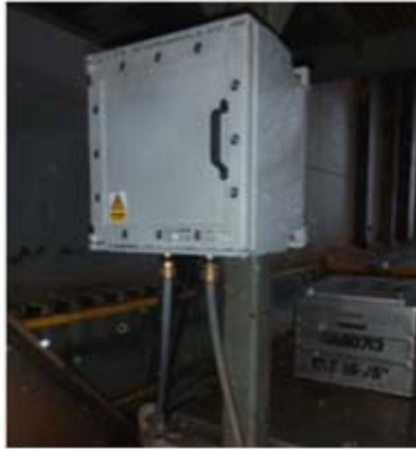
Figure 10 – 3-Axis Precision Accelerometer in EExd Housing
