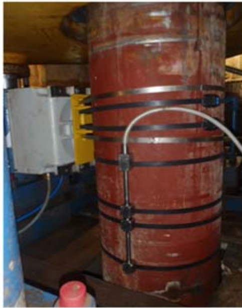
Figure 11 – Dynamic Curvature Sensor Measuring Fatigue Accumulation on Tension Joint
