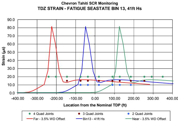
**Figure 9 – 100 yr TDZ Strain vs Monitoring Locations**
