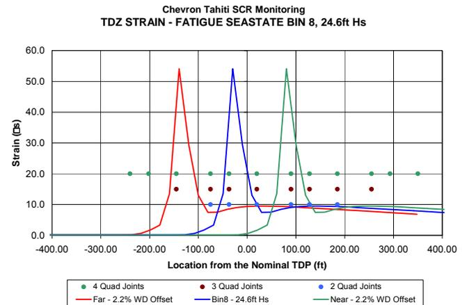
**Figure 8 – 10 yr TDZ Strain vs Monitoring Locations**
