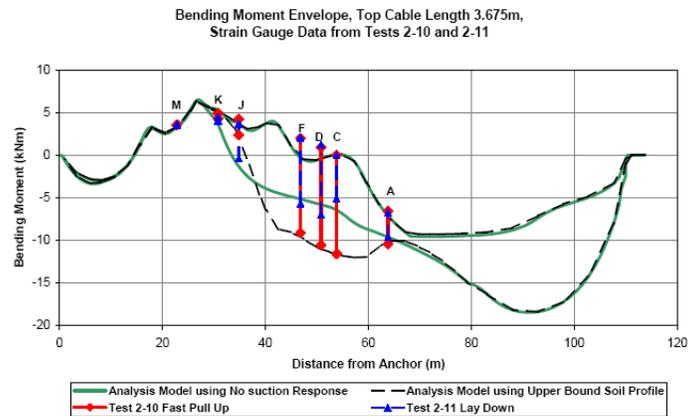
**Figure 20 –Soil Suction Model Calibration, STRIDE JIP**
