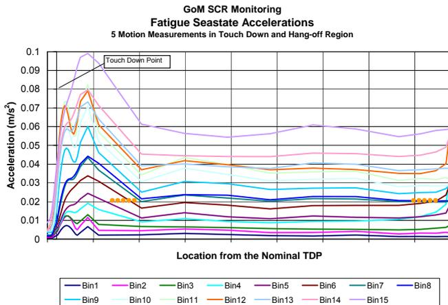
Figure 15 – Riser Accelerations for a Typical GoM SCR
