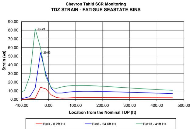
**Figure 6 – Touch Down Region Strain Distribution**
