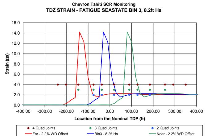
**Figure 7 – 1 yr TDZ Strain vs Monitoring Locations**
