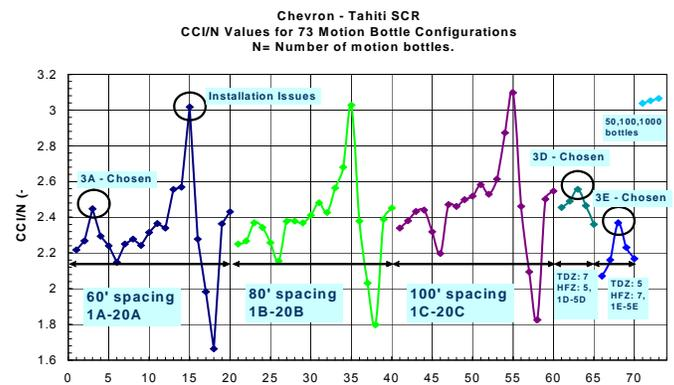
**Figure 5 – Configuration Clarity Indices for 73 Motion Bottle Arrangements**
