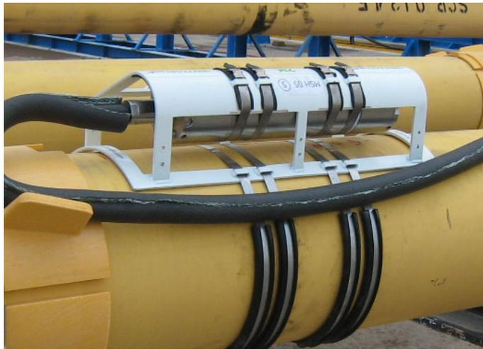
**Figure 2 –INTEGRIPod Motion Sensor Installed on SCR Joint**
