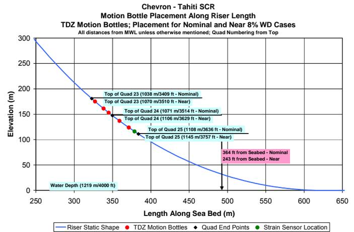
**Figure 10 – Optimized (Final) Motion Bottle Location**
