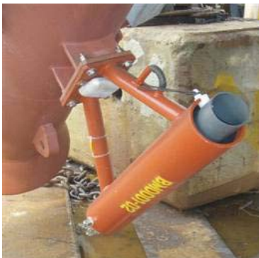
Permanently installed pod holders allow pods to be installed by ROV or divers
