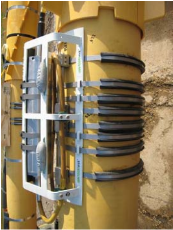
INTEGRistick™ dynamic curvature sensor and motion sensor package
