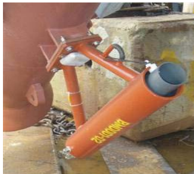
Permanently installed pod holders on chain stoppers to allow pods to be installed by ROV or divers
