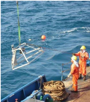
Seabed deployment of 75kHz ADCP
