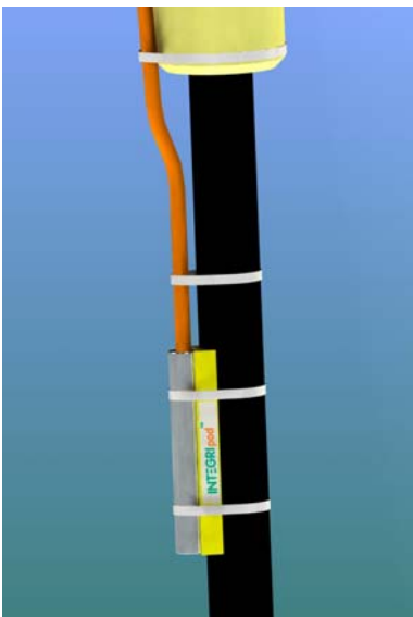
FLEXASSURE™ lower pod attached to the riser below the bend stiffener
